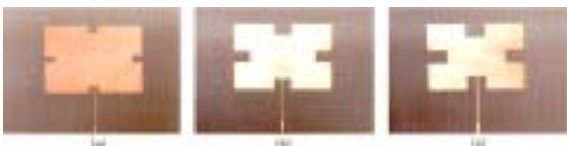
Fig.2. 1st iteration Koch fractal island microstrip patch antenna with different fractal factor:(a) 1/10 iteration factor (b) 1/6 iteration factor (c) 1/5 iteration factor
