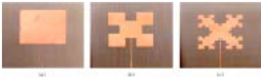
Fig. 1. Koch fractal island microstrip antennas for iteration factor 1/4
