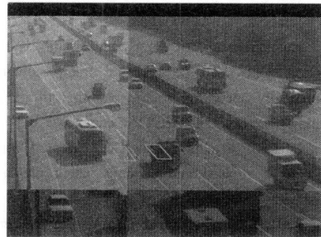
(b) Extract the restored image from the hemisphere database and marked detection zone which calculated with changing pan, tilt angle.
