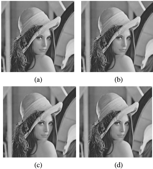
그림 10. 제한한 경계처리에 의한 영상결과 (a) 원영상 (b) SE-SE(48.1308dB) (c) EE-EE(38.9297dB) (d) EE-SE (39.3947dB) Fig 10. Image result by proposed boundary processing (a) original image (b) SE-SE (48.1308dB) (c) EE-EE (38.9297dB) (d) EE-SE(39.3947dB)
