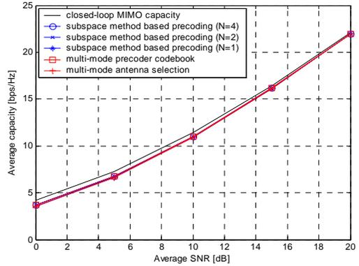
Fig. 2. Capacity comparison between precoding schemes in loosely correlated channels when  $n_T = n_R = 4$ .
