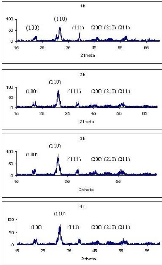
Fig. 2. X-ray diffraction patterns for PZT powders calcined at 900°C as a function of calcining time
