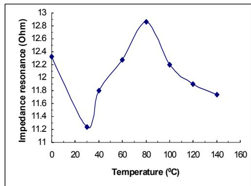
Fig. 5. Impedance resonance as a function of temperature
