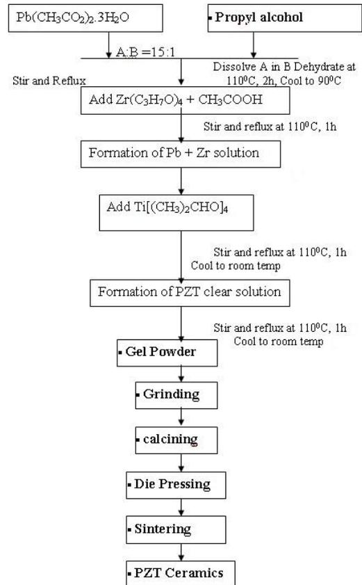
Fig. 1. Flow diagram for the preparation of PZT
