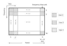
Fig. 1. OFDMA system in frequency-time axis
