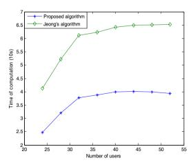
Fig. 5. Calculation complexity according to the number of users
