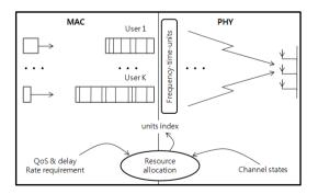
Fig. 2. Procedure of cross-layer resource allocation algorithm
