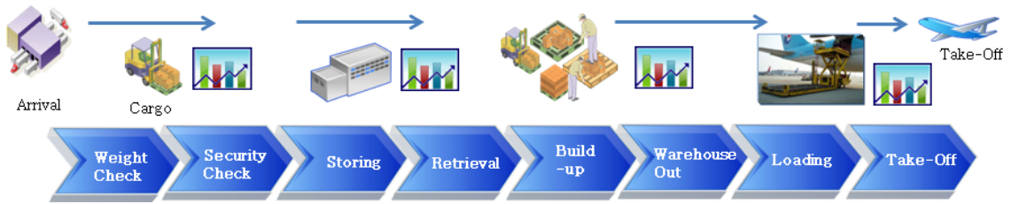
Fig. 1. Air-cargo movement process (export).
