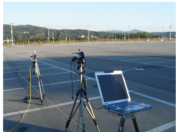
Fig. 5. Measurement set-up of interference between SDMB and UWB
