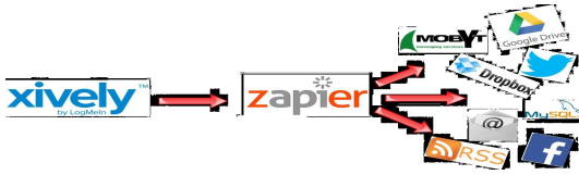
Fig. 8. The Zapier service acts as a bridge between Xively triggers and applications.
