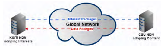
Fig. 7. NDN ping test procedure between KISTI and CSU testbeds
