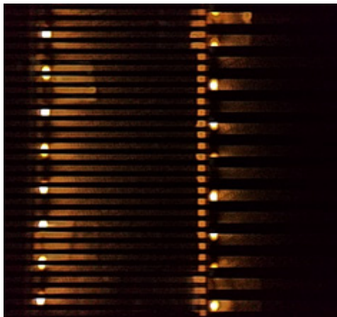
Fig. 7. F1=1kHz, F2= 1.5kHz, d=6cm FOV=90 on rolling shutter image sensor.
