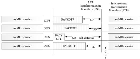
(b) LBT Type A with self-deferral to combat RF leakage
