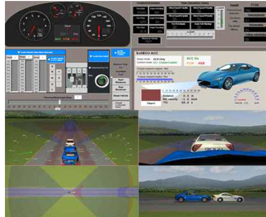
Fig. 10. Virtual vehicle based environment build
